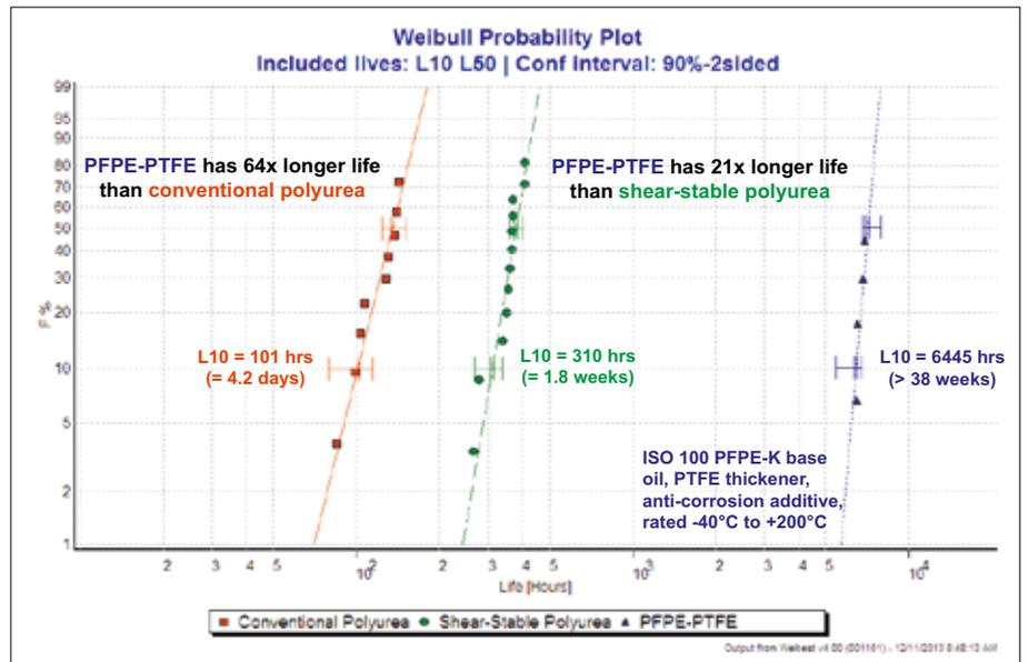
Results from SKF ROF+ bench bearing life test using 6204 bearings at 10,000 rpm at 177 °C.
